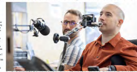
Above: MetroHealth ALT Lab's Blake Perkins works with David Pedrick, patient and IT consultant. Pedrick is using a SmartLink, a top and bottom extended device for computer access — a device that Pedrick uses to operate his computer and run his IT business. Below: Perkins works with Josh Schaefer, patient and ALT Lab consultant. Schaefer is using a SmartLink adaptive pointing device to pick up a glass for independent dining. Photos courtesy of Cleveland VCS Center.
