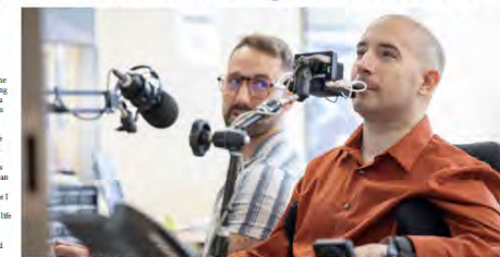
Above: MetroHealth ALT Lab's Blake Perkins works with David Pedrick, patient and IT consultant. Pedrick is using a SmartLink, a top and self-directed device for computer access — a device that Pedrick wears to operate his computer and run his IT business. Below: Perkins works with Josh Schaeffer, patient and ALT Lab consultant. Schaeffer is using a SmartLink adaptive pointing device to pick up a glass for independent dining. Photos courtesy of Cleveland VCU Center.
