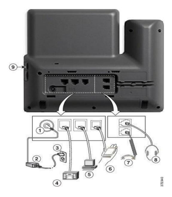
To set up the PC. Plug the cable into port 5 on the phone and into the network port on the PC.
